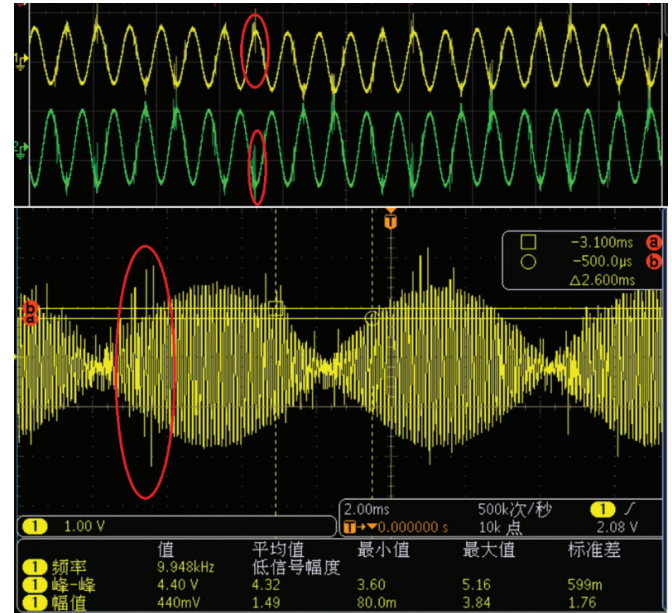
Figure 6. A SIN/COS coupled IGBT disturbance.
