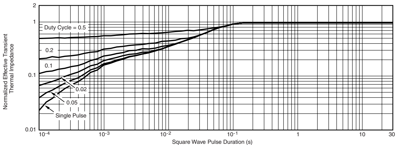
Normalized Thermal Transient Impedance, Junction-to-Case
