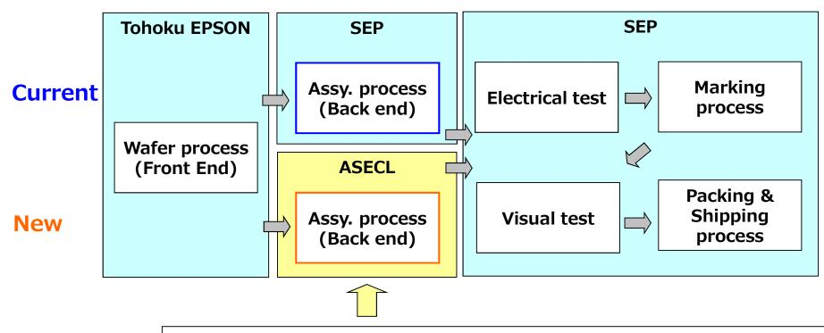
·Assembly process (plant) change Wafer process, Test process, Marking process, Shipping process: no change
