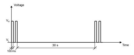
Figure 7: GPIO pin progress for registered roaming NB-IoT
