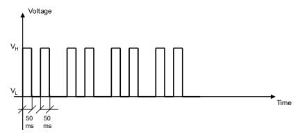
Figure 6: GPIO pin progress for registered roaming 3G
