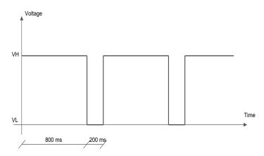
Figure 9: GPIO pin progress for data transmission roaming
