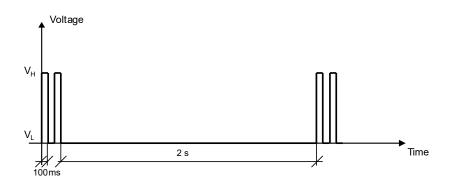
Figure 5: GPIO pin progress for registered roaming 2G
