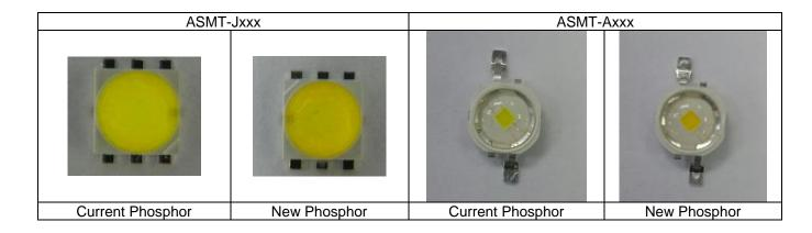
The color spectrum is different between the new phosphor and current phosphor as illustrated below.
