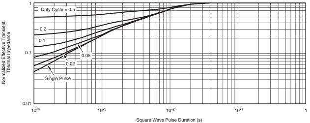
Normalized Thermal Transient Impedance, Junction-to-Case
