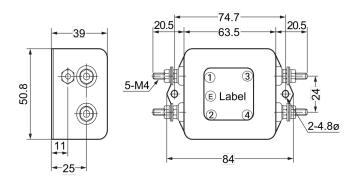
**General Information** Series GT Style Metal Box Description Noise Filters RoHS With Exemptions SCIP Number 178c3d71-76e7-4e48-aa60-e3285a8f7efd Notes DC Available. Miscellaneous 35 K Self-Temperature Rise Max. Lead Screw Terminals Terminal Type Screw
