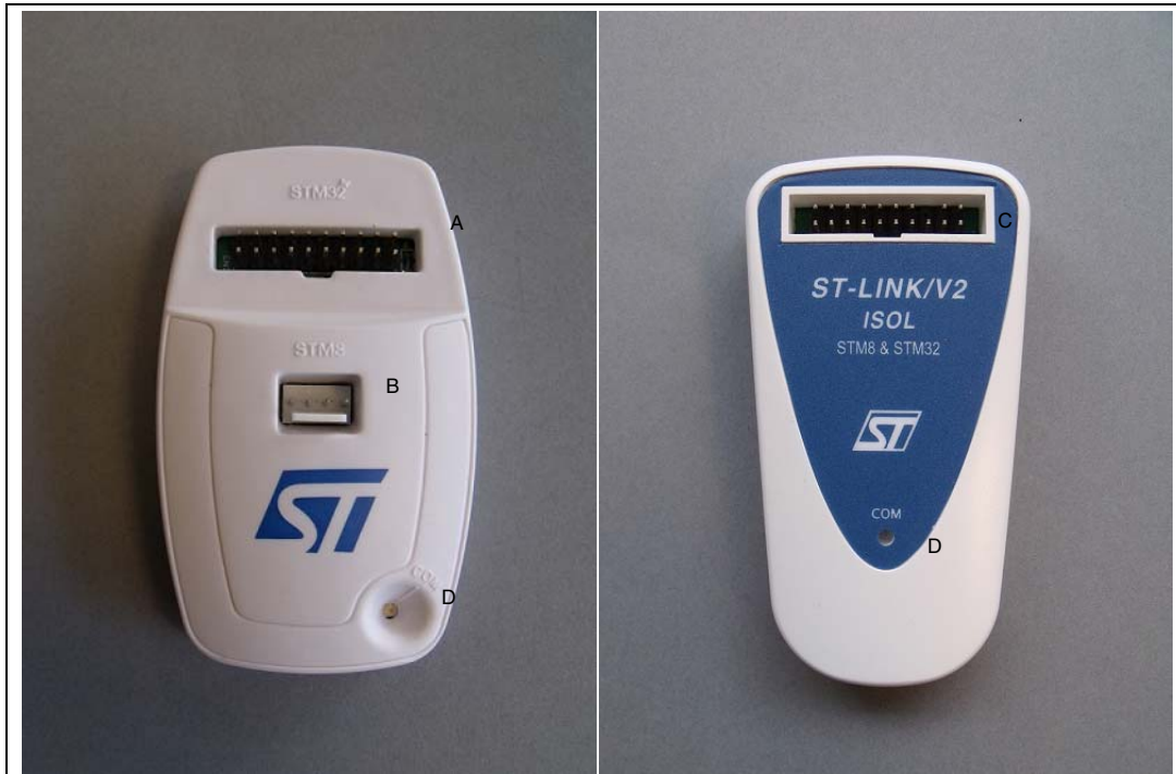
Figure 4. Connectors of the ST-LINK/V2 (on the left) and of the ST-LINK/V2-ISOL (on the right)
