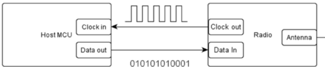
Figure 28. GPIO Connections between the Radio and the Host MCU (Direct TX)
