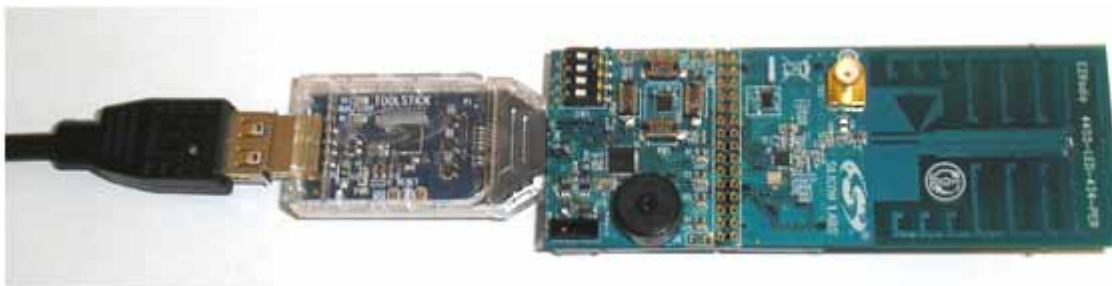
Figure 2. How to Connect the RFStick to the PC
