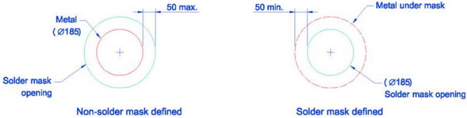
Solder mask detail (not to scale)
