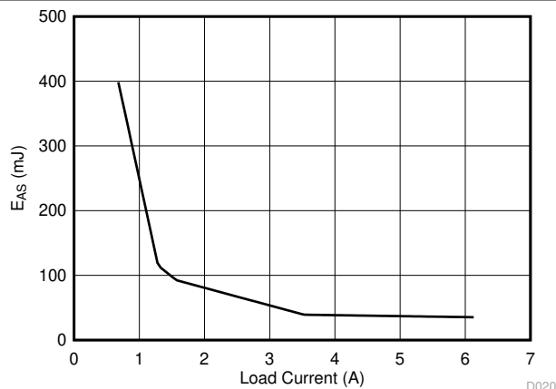
Figure 8-8. Maximum Energy Dissipation ( E_{AS} ) Allowed T_{J\_start} = 125^{\circ}\text{C} - Single Pulse, One Channel
