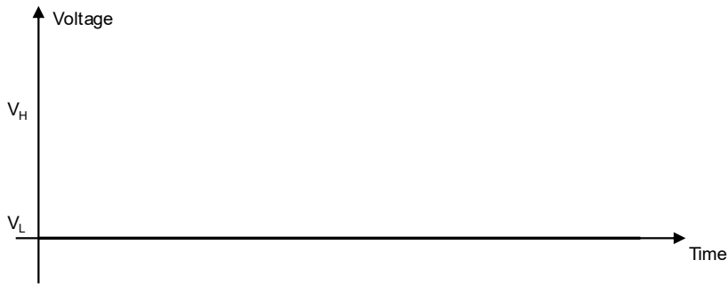
Figure 1: GPIO pin progress for no service
